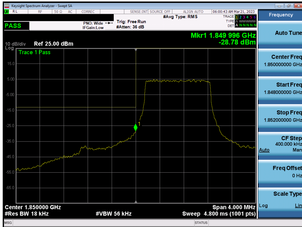
Plot 7-42. Lower Band Edge Plot (LTE Band 2 – 1.4MHz QPSK – Full RB)
