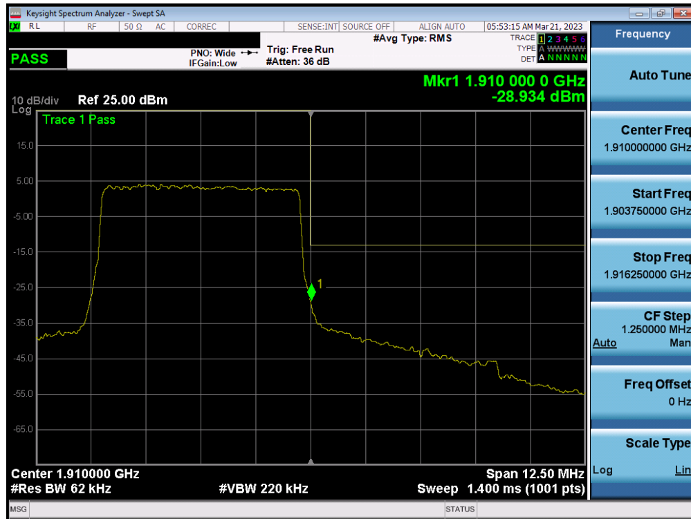
Plot 7-36. Upper Band Edge Plot (LTE Band 2 - 5MHz QPSK – Full RB)
