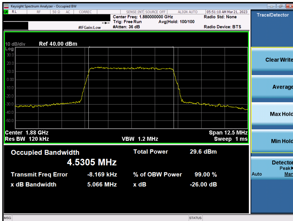
Plot 7-7. Occupied Bandwidth Plot (LTE Band 2 - 5MHz QPSK - Full RB)
