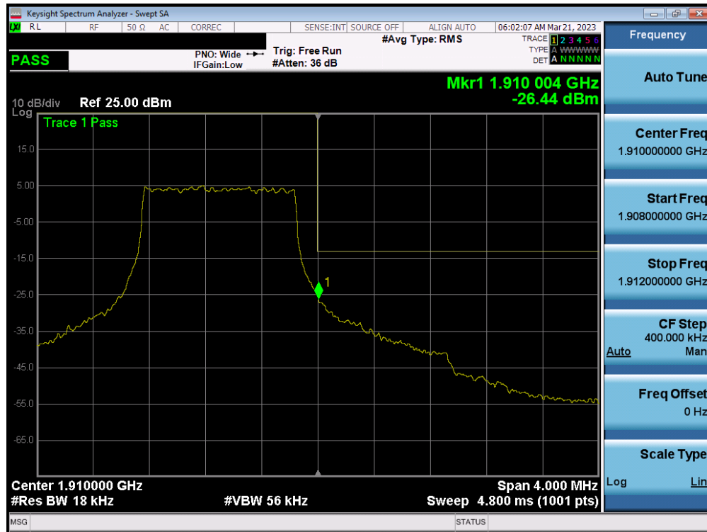
Plot 7-44. Upper Band Edge Plot (LTE Band 2 – 1.4MHz QPSK – Full RB)
