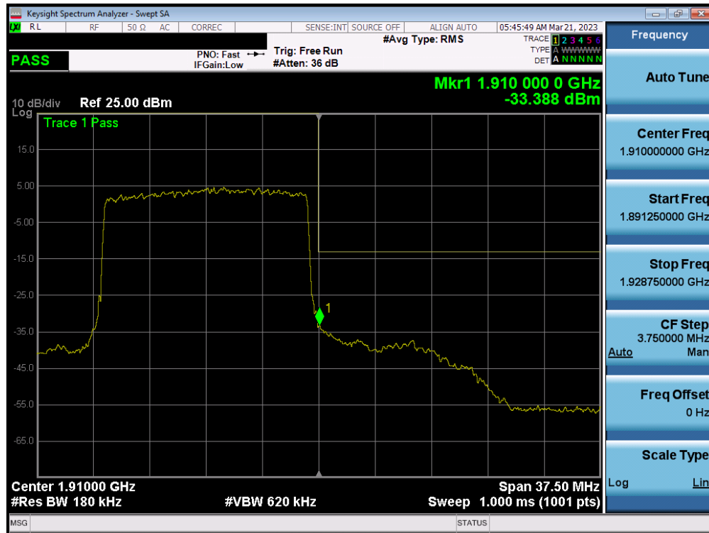
Plot 7-28. Upper Band Edge Plot (LTE Band 2 - 15MHz QPSK – Full RB)
