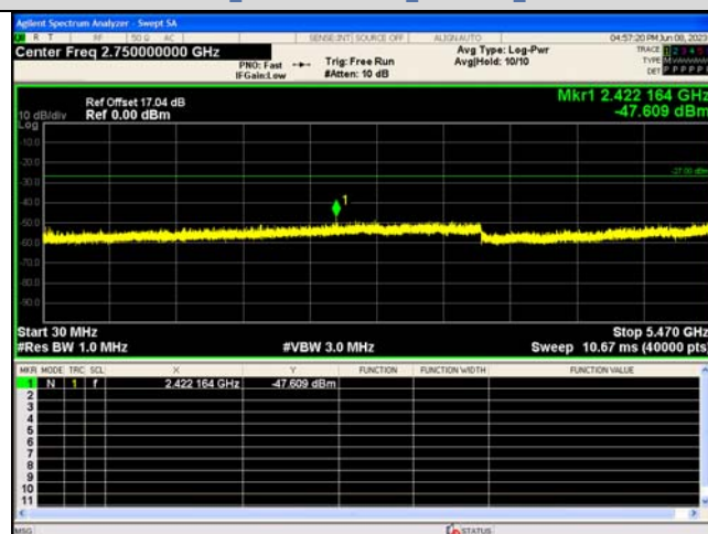
Spurious Emission:30.0~5470 MHz IEEE 802.11n_Channel 140_20MHz_Antenna 0
