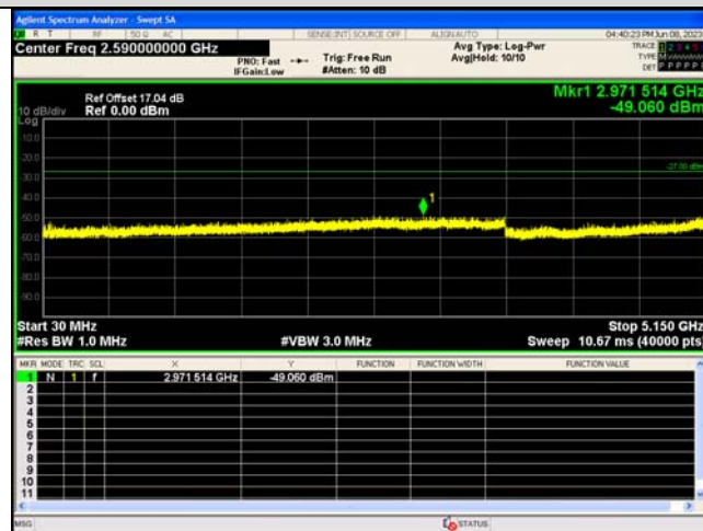
Spurious Emission:30.0~5150 MHz IEEE 802.11n_Channel 62_40MHz_Antenna 0
