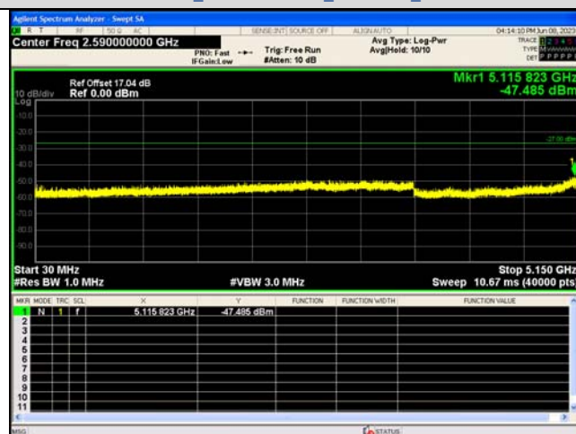
Spurious Emission:30.0~5150 MHz IEEE 802.11n_Channel 46_40MHz_Antenna 0
