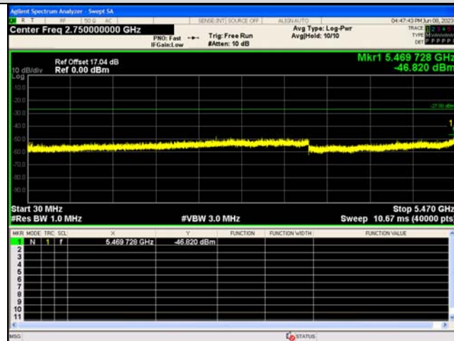
Spurious Emission:30.0~5470 MHz IEEE 802.11a_Channel 120_20MHz_Antenna 0
