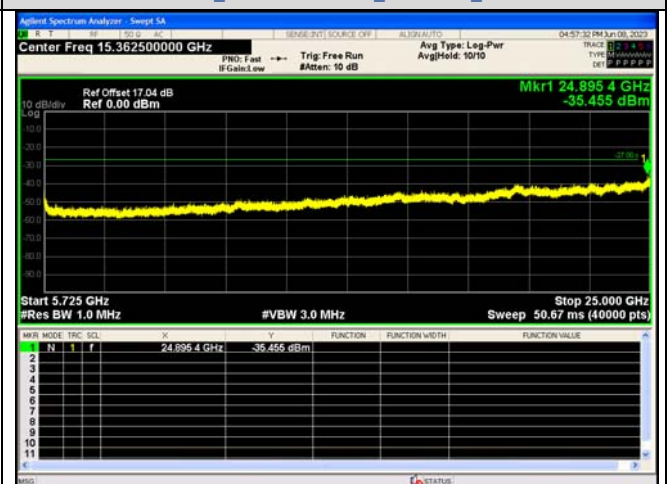
Spurious Emission:5725~25000.0 MHz IEEE 802.11n_Channel 140_20MHz_Antenna 0
