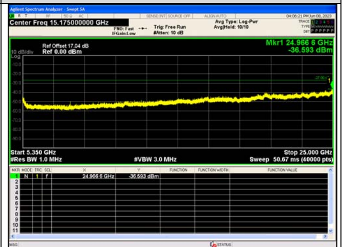
Spurious Emission:5350~25000.0 MHz IEEE 802.11n_Channel 48_20MHz_Antenna 0
