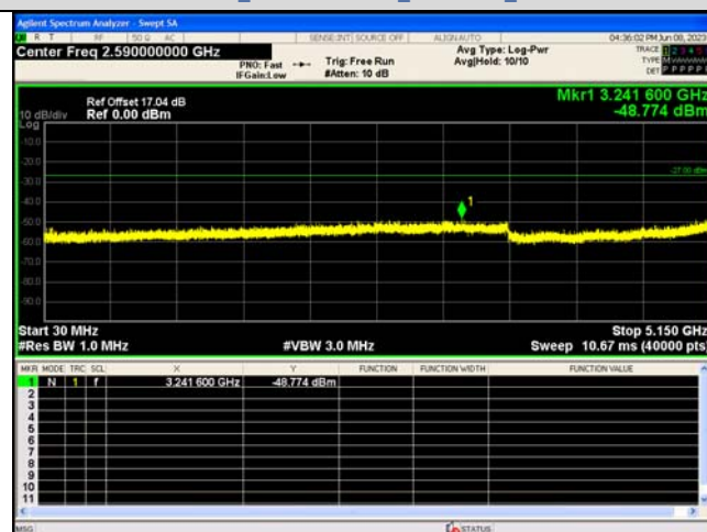
Out Of Band Emission IEEE 802.11n_Channel 56_20MHz_Antenna 0
