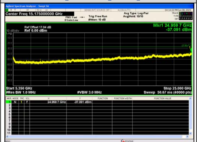
Spurious Emission:5350~25000.0 MHz IEEE 802.11n_Channel 46_40MHz_Antenna 0
