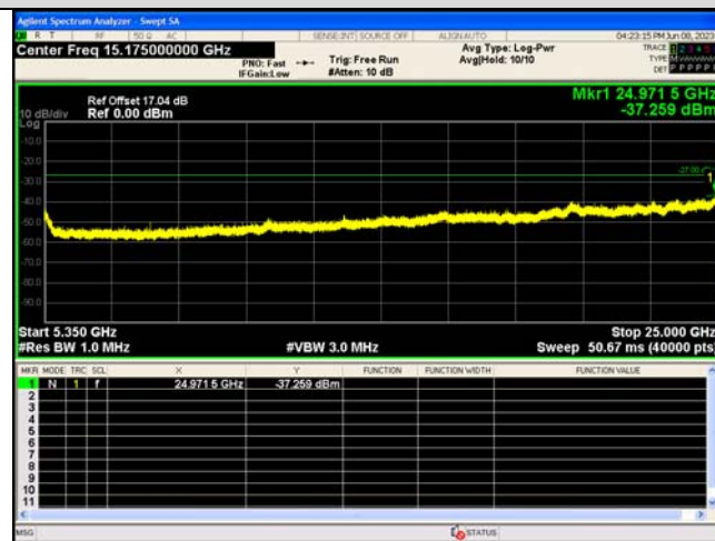
Spurious Emission:5350~25000.0 MHz IEEE 802.11a_Channel 56_20MHz_Antenna 0
