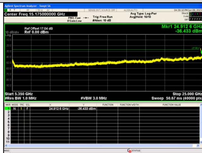
Spurious Emission:5350~25000.0 MHz IEEE 802.11n_Channel 54_40MHz_Antenna 0
