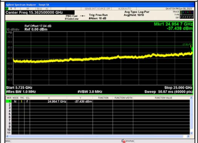
Spurious Emission:5725~25000.0 MHz IEEE 802.11a_Channel 120_20MHz_Antenna 0
