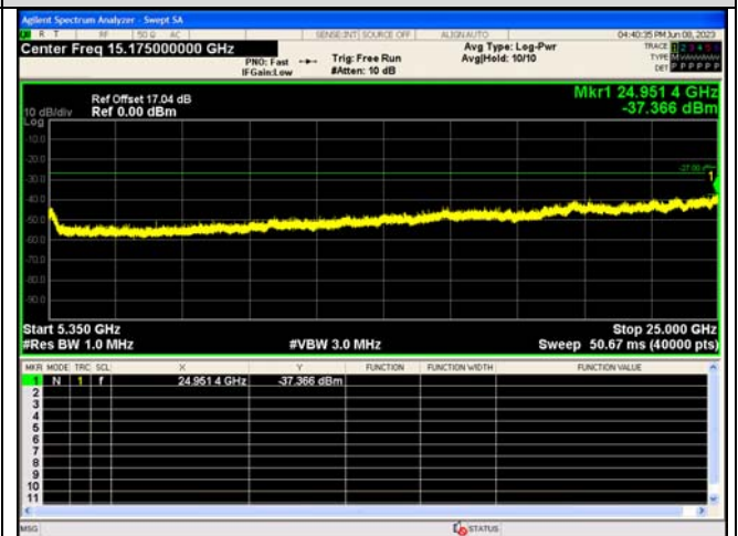
Spurious Emission:5350~25000.0 MHz IEEE 802.11n_Channel 62_40MHz_Antenna 0
