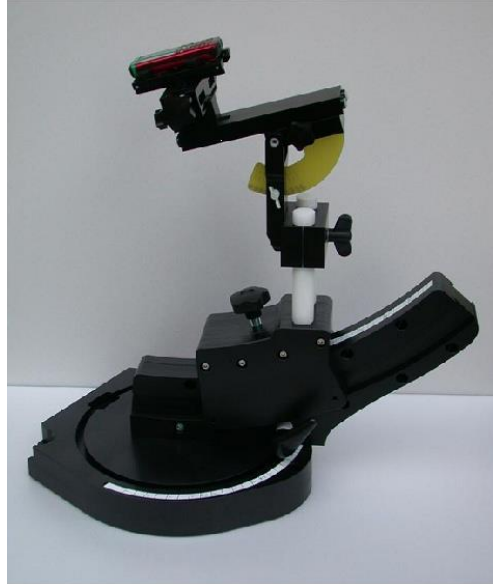
Device holder supplied by SPEAG
