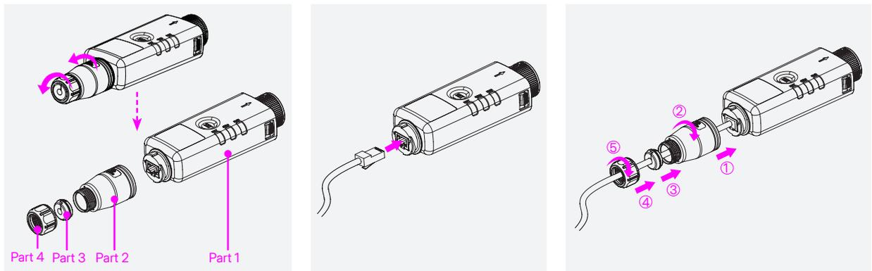
**Step 4** Remove the DTS port cover on the bottom of the inverter.
