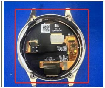
The antenna is Metal frame antenna.
