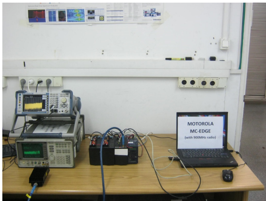
Figure 6. Conducted Emission Test from Antenna Ports
