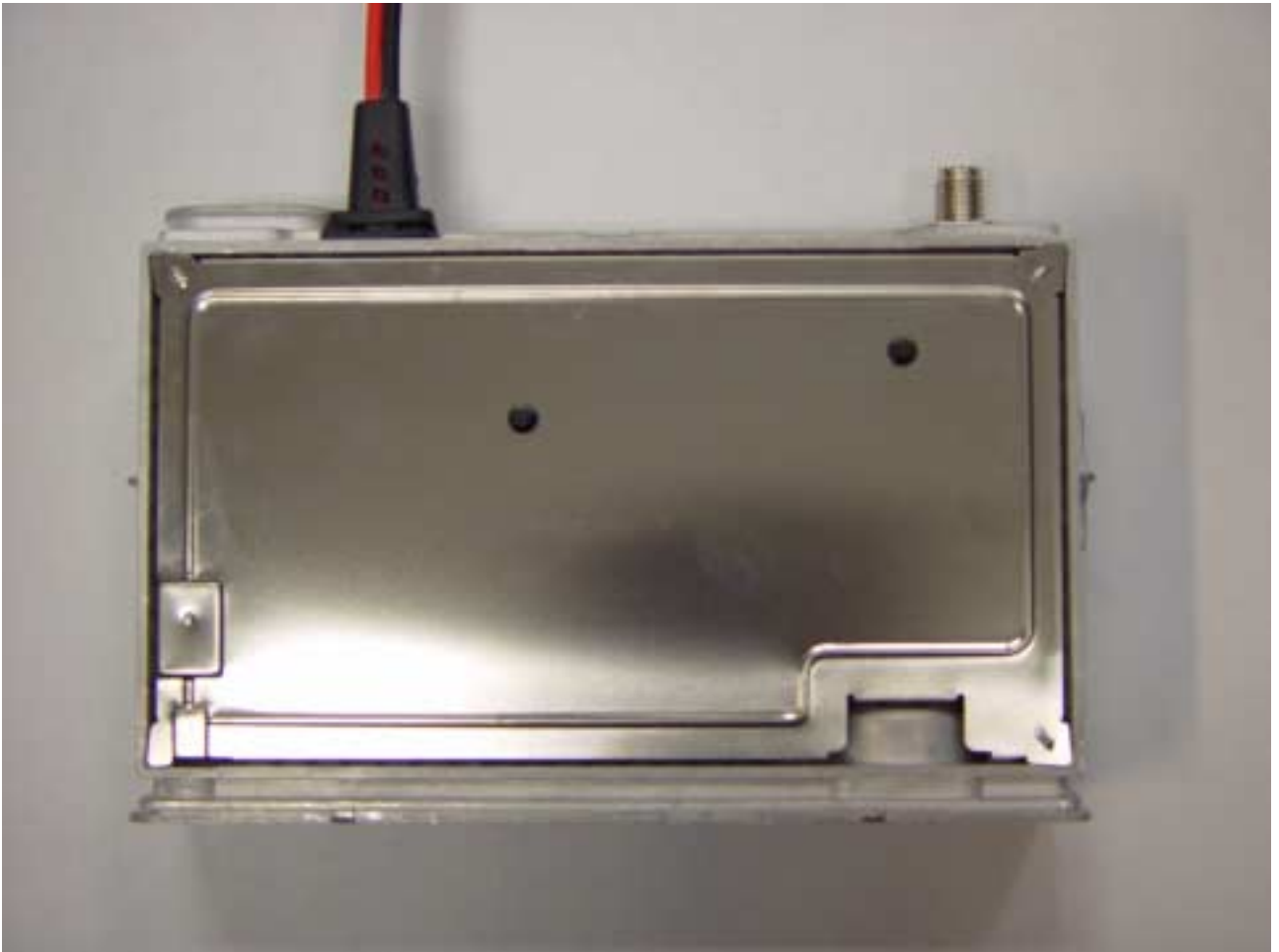
TOP VIEW OF RADIO WITH PLASTIC HOUSING REMOVED
