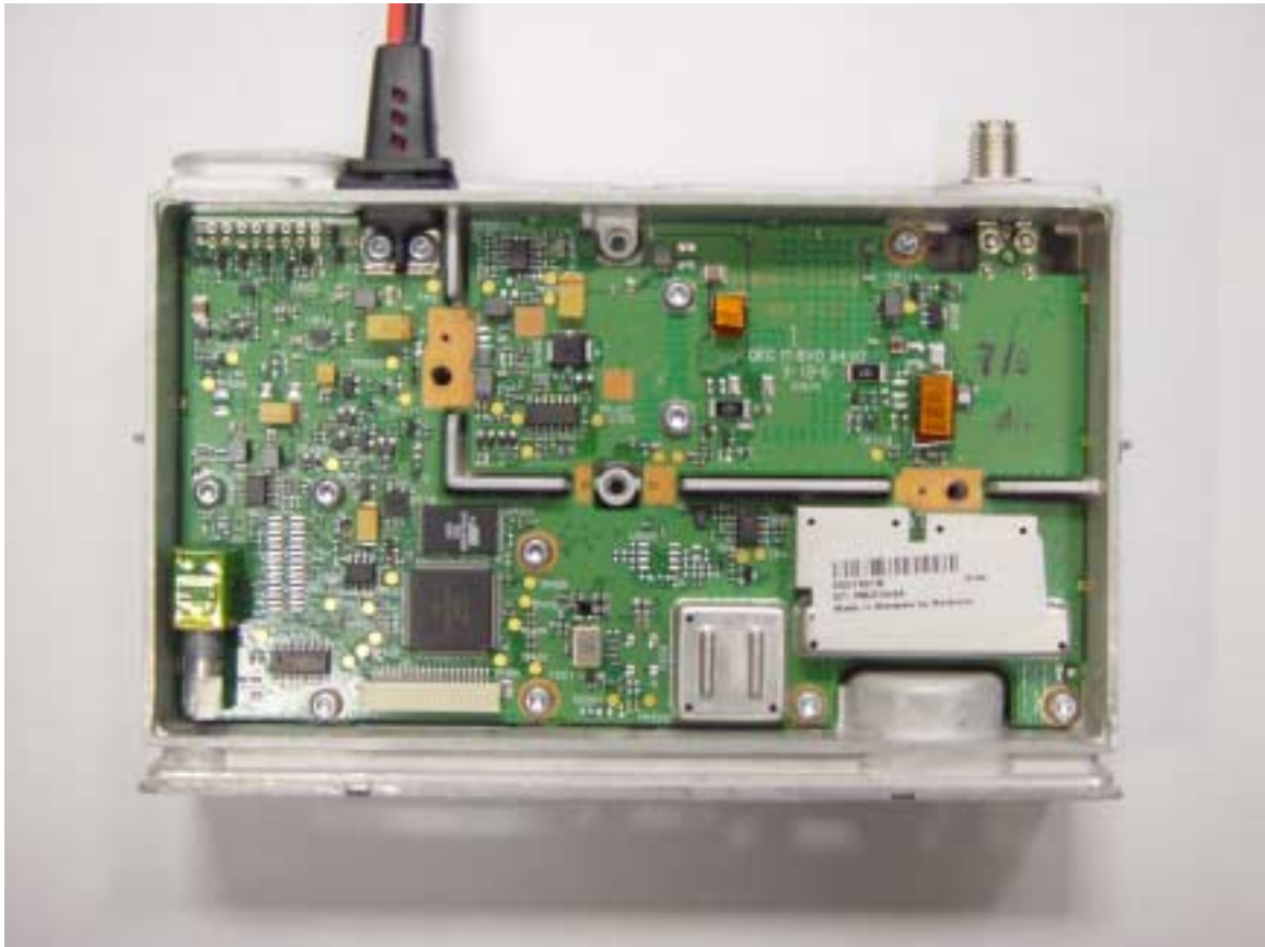
TOP VIEW OF RADIO WITH PA SHIELD REMOVED
