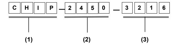
(1) Product type: PCB Antenna(2) Center Frequency: 2450MHz
