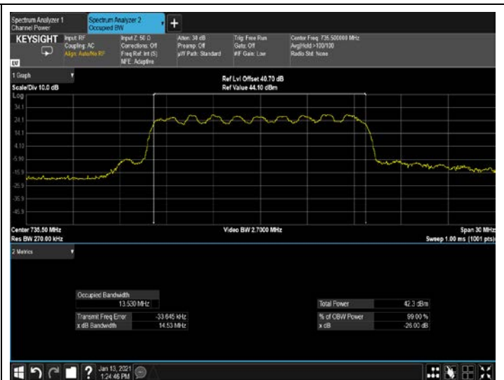
Figure 286: 16QAM 15MHz B.W; 735.5MHz, 30kHz OUTPUT
