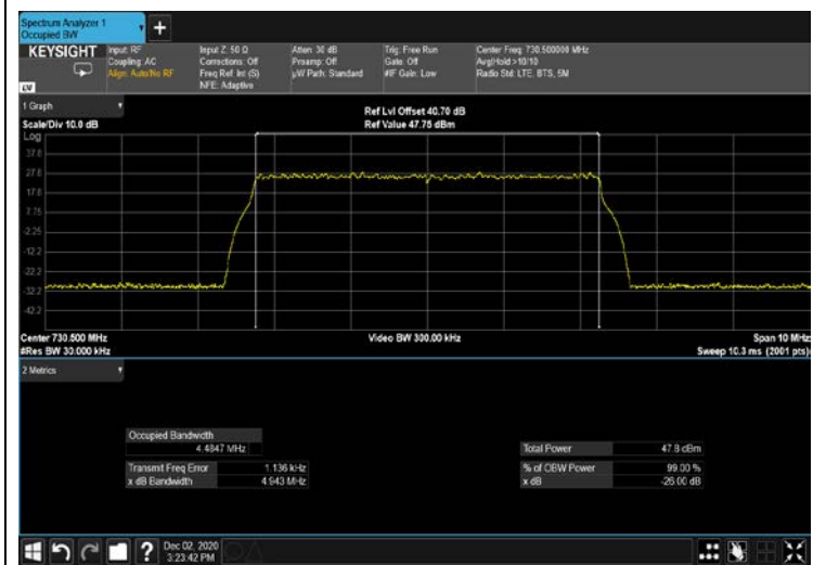
Figure 336: 64QAM 5MHz B.W; 730.5MHz Input 4G
