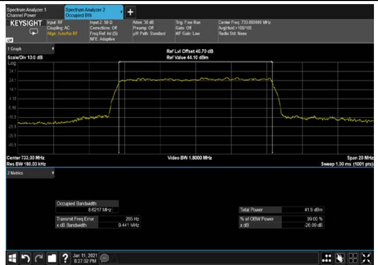
Figure 294: 64QAM 10MHz B.W; 733.0MHz, 30kHz OUTPUT
