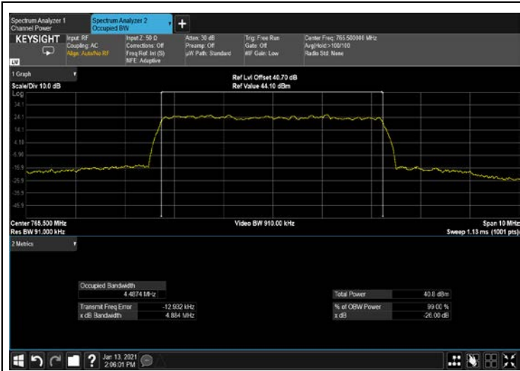
Figure 291: 64QAM 5MHz B.W; 765.5MHz, 15kHz OUTPUT
