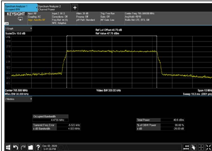
Figure 359: 64QAM 5MHz B.W; 765.5MHz output 4G
