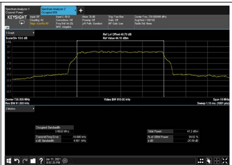
Figure 288: 64QAM 5MHz B.W; 730.5MHz, 30kHz OUTPUT
