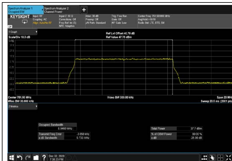
Figure 340: 64QAM 10MHz; 751.5MHz Input 4G
