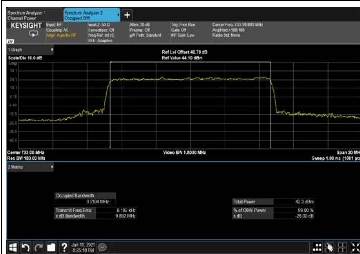
Figure 293: 64QAM 10MHz B.W; 733.0MHz, 15kHz OUTPUT
