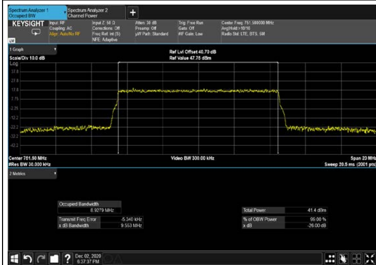
Figure 361: 64QAM 10MHz; 751.5MHz output 4G
