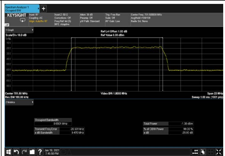
Figure 254: 256QAM 10MHz B.W; 751.5MHz, 30kHz INPUT
