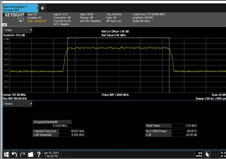
Figure 253: 256QAM 10MHz B.W; 751.5MHz, 15kHz INPUT
