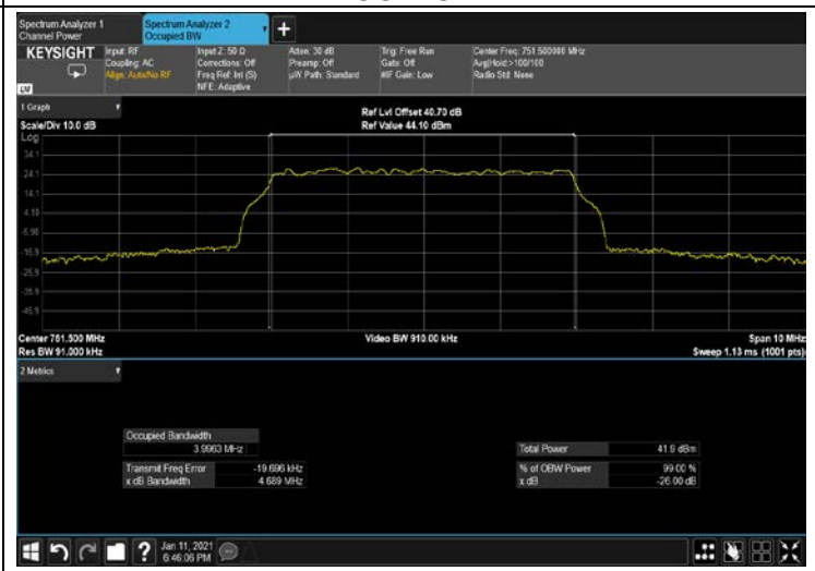
Figure 290: 64QAM 5MHz B.W; 751.5MHz, 30kHz OUTPUT
