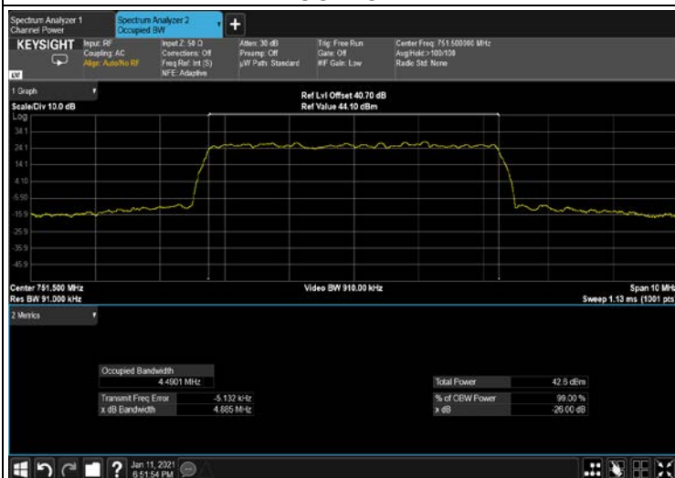
Figure 289: 64QAM 5MHz B.W; 751.5MHz, 15kHz OUTPUT
