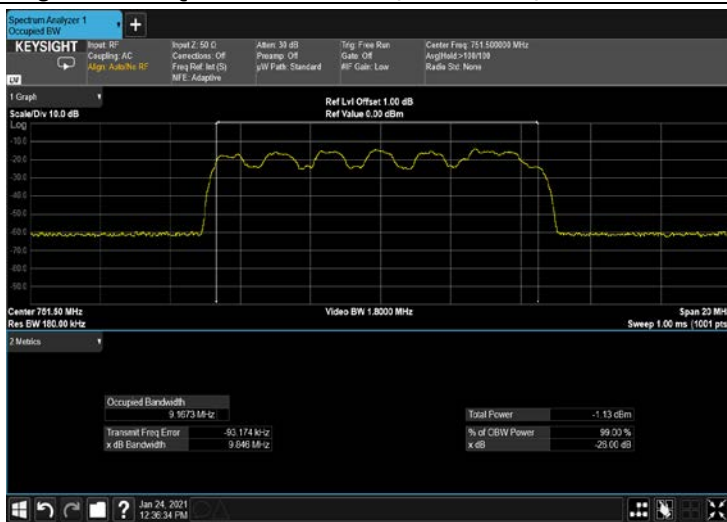
Figure 267: QPSK 10MHz B.W; 751.5MHz, 15kHz INPUT
