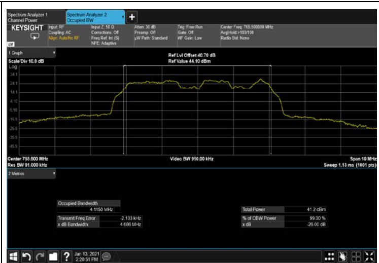
Figure 320: QPSK 5MHz B.W; 765.5MHz, 30kHz OUTPUT
