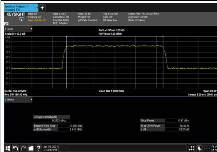
Figure 255: 256QAM 10MHz B.W; 763.0MHz, 15kHz INPUT
