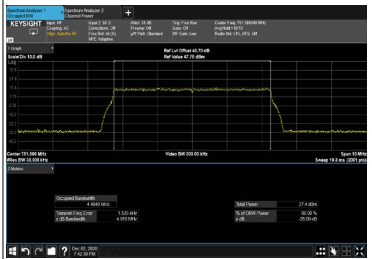
Figure 337: 64QAM 5MHz B.W; 751.5MHz Input 4G
