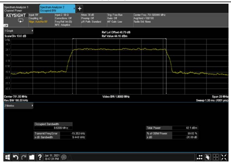
Figure 296: 64QAM 10MHz B.W; 751.5MHz, 30kHz OUTPUT
