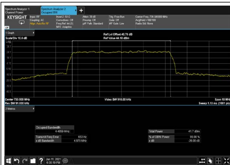
Figure 287: 64QAM 5MHz B.W; 730.5MHz, 15kHz OUTPUT
