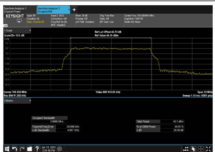
Figure 292: 64QAM 5MHz B.W; 765.5MHz, 30kHz OUTPUT
