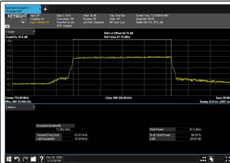
Figure 363: 64QAM 15MHz B.W; 735.5MHz output 4G
