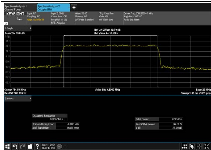
Figure 295: 64QAM 10MHz B.W; 751.5MHz, 15kHz OUTPUT
