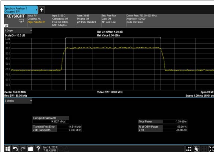
Figure 251: 256QAM 10MHz B.W; 733.0MHz, 15kHz INPUT
