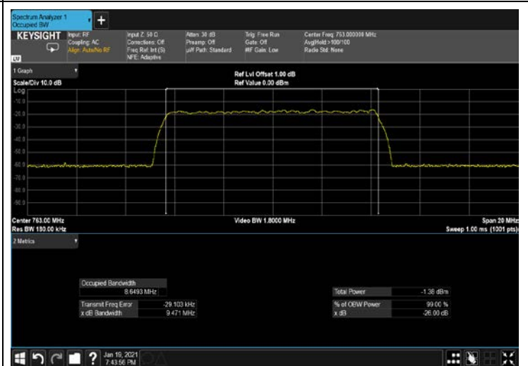
Figure 256: 256QAM 10MHz B.W; 763.0MHz, 30kHz INPUT
