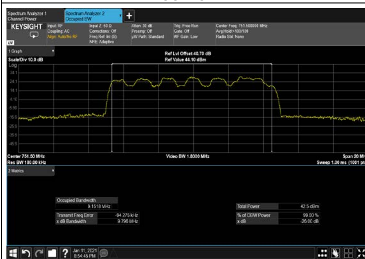
Figure 323: QPSK 10MHz B.W; 751.5MHz, 15kHz OUTPUT
