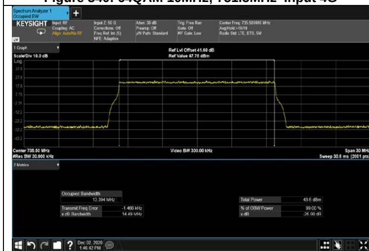
Figure 342: 64QAM 15MHz B.W; 735.5MHz Input 4G
