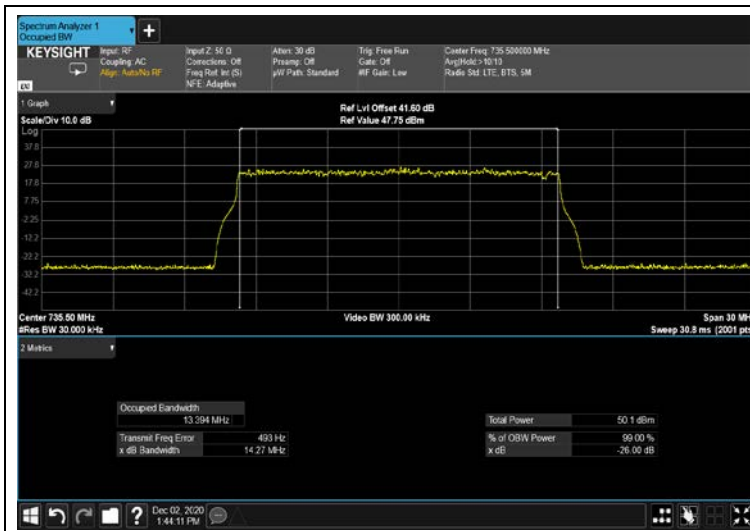
Figure 335: 16QAM 15MHz B.W; 735.5MHz Input 4G
