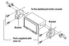
When mounting this unit to the preinstalled brackets of your car, use the mounting screws (2) in the appropriate screw holes based on your car: T for TOYOTA and N for NISSAN.
