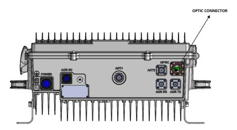
Optical cables should be inserted into Optic Port outside of N2ROU.
