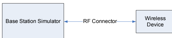
Figure 9-1 Power Measurement Setup
