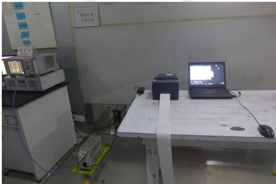
CONDUCTED EMISSION TEST SETUP
