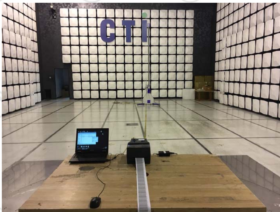
RADIATED EMISSION TEST SETUP
