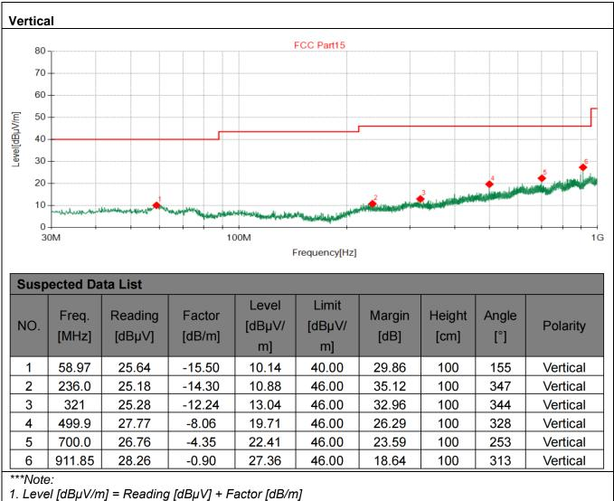
2. Margin [dB] = Limit [dB $\mu$ V/m] - Level [dB $\mu$ V/m]
