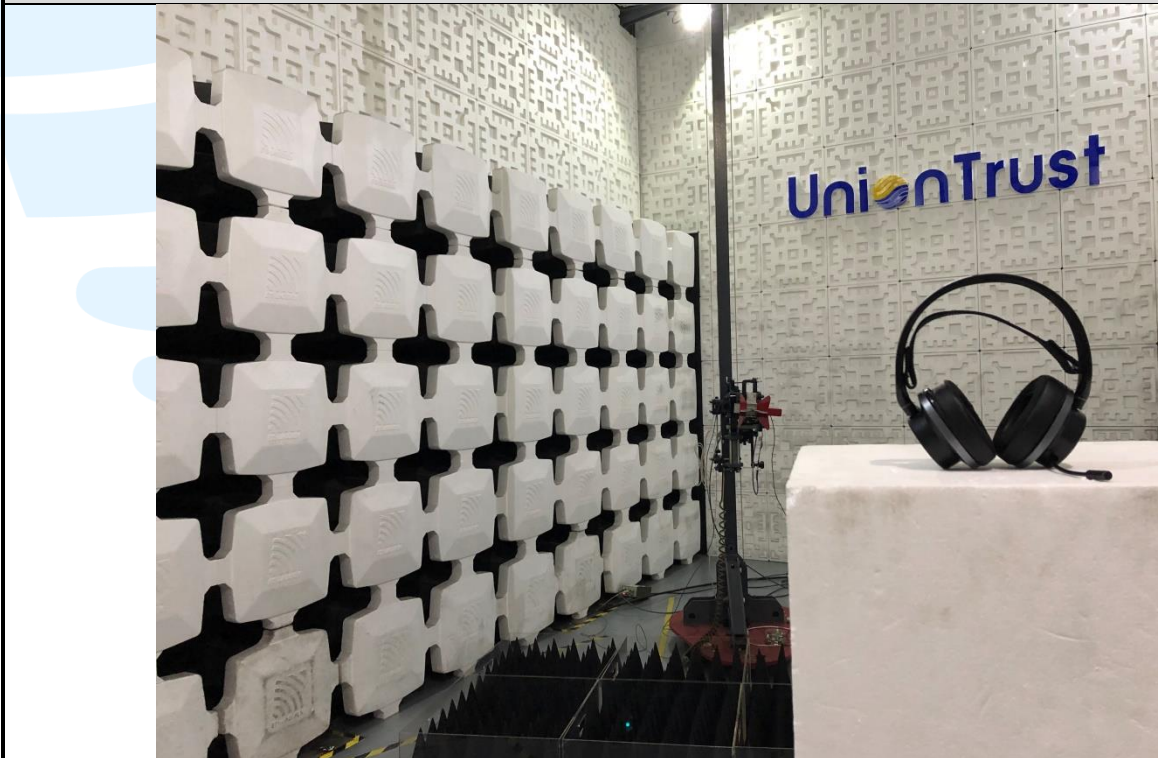
Radiated emission Test Setup (Above 1 GHz)
