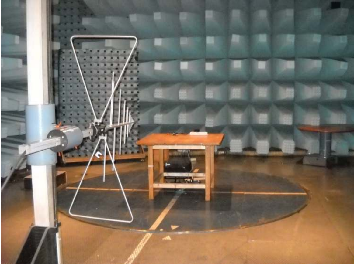
Figure 0-2: Radiated emission test below 1 GHz
