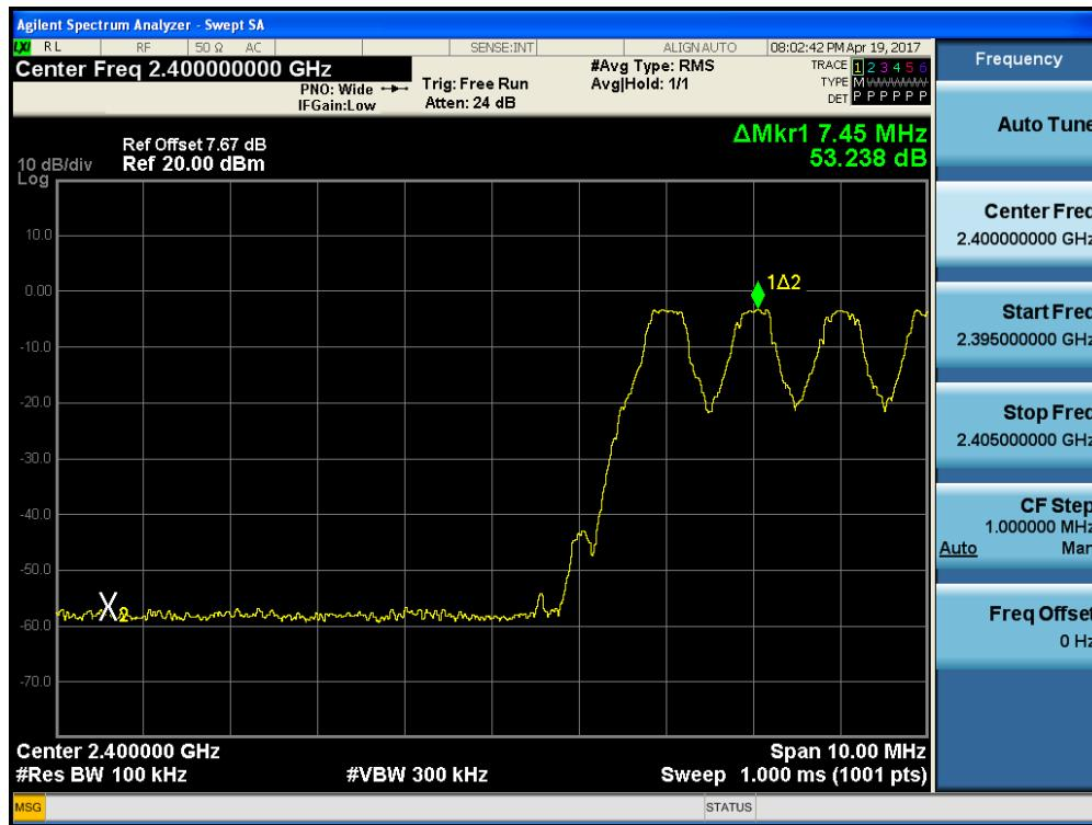
Test Plots with hopping (GFSK)
