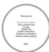
1 Temp./hum. offset: Set temperature offset from 0~10°C, the temperature offset would be 0.5°C increase or decrease; Set humidity offset from 0~100%, the humidity offset would be 1% increase or decrease.
