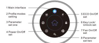
Rotation the first ring to select the parameter setting, and press the panel to confirm the selection.
