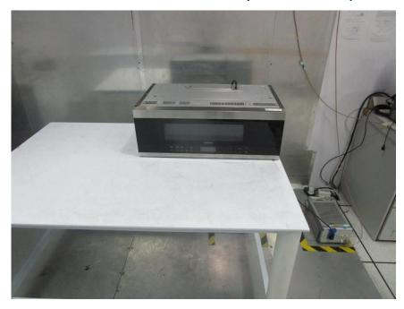
1.2 Radiated Emissions (30MHz-1GHz) Test Setup
