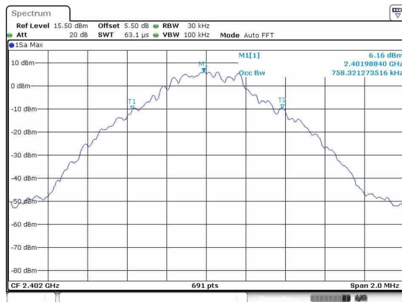
99% Occupied Bandwidth Plot on Channel 00
