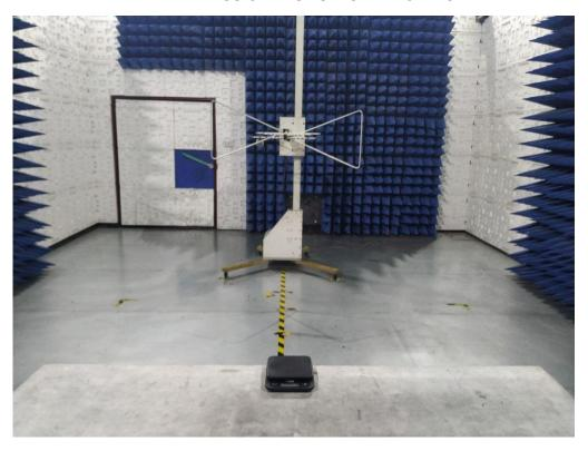
RADIATED EMISSION TEST SETUP ABOVE 1GHZ
