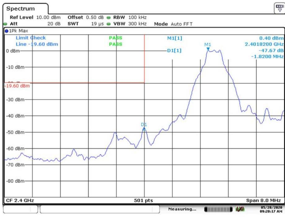
**Band Edge, Right Side**
