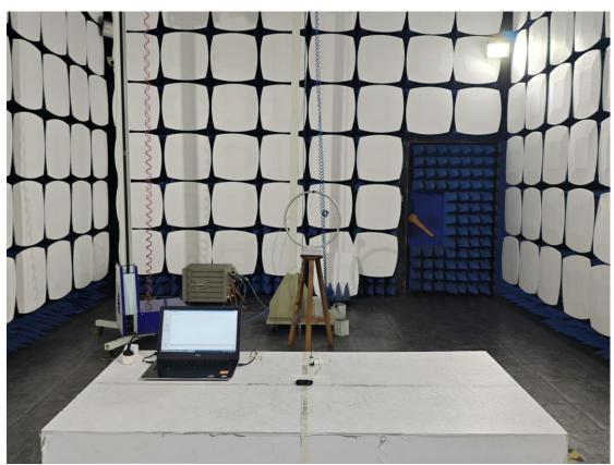
3. Radiated emission (9KHz-30MHz)
