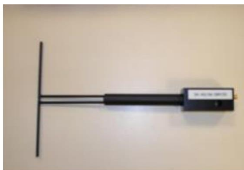
Figure 1 – Satimo COMOSAR Validation Dipole
