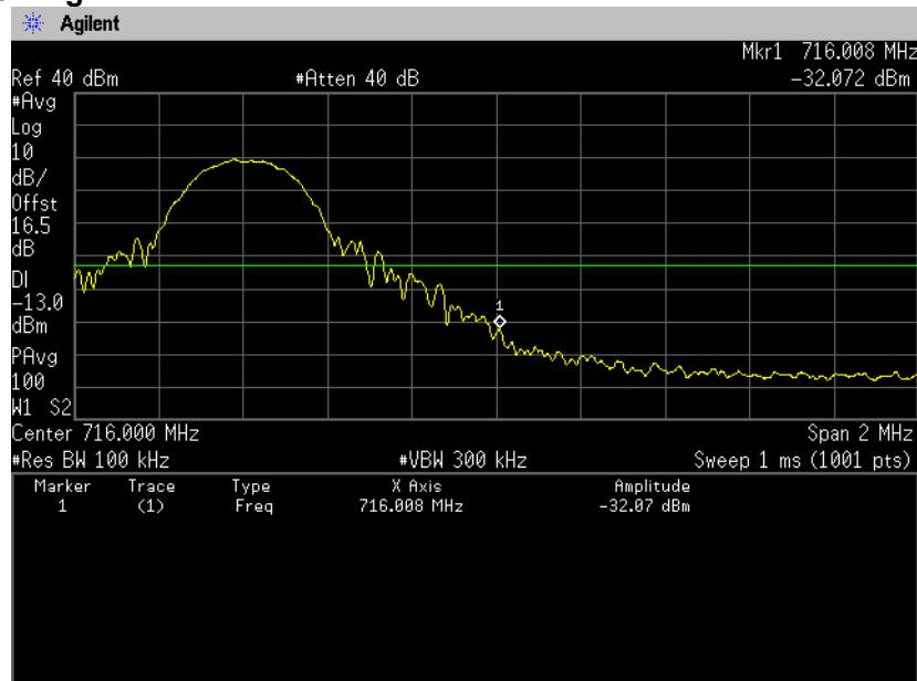
**16QAM, BW 10MHz, RB50-0****Channel: Low**
