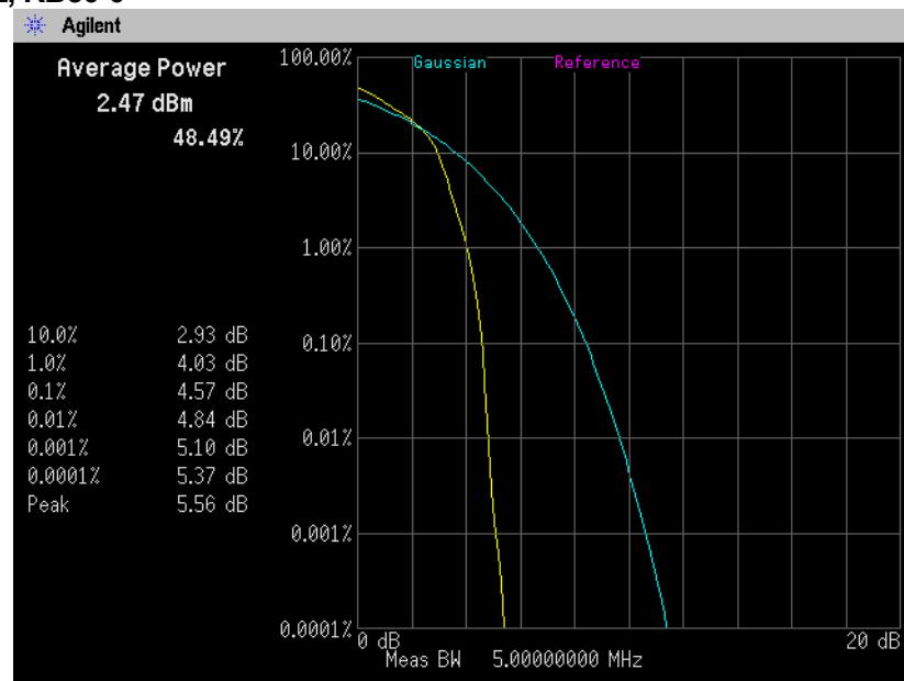
**16QAM, BW 5MHz, RB25-0**
