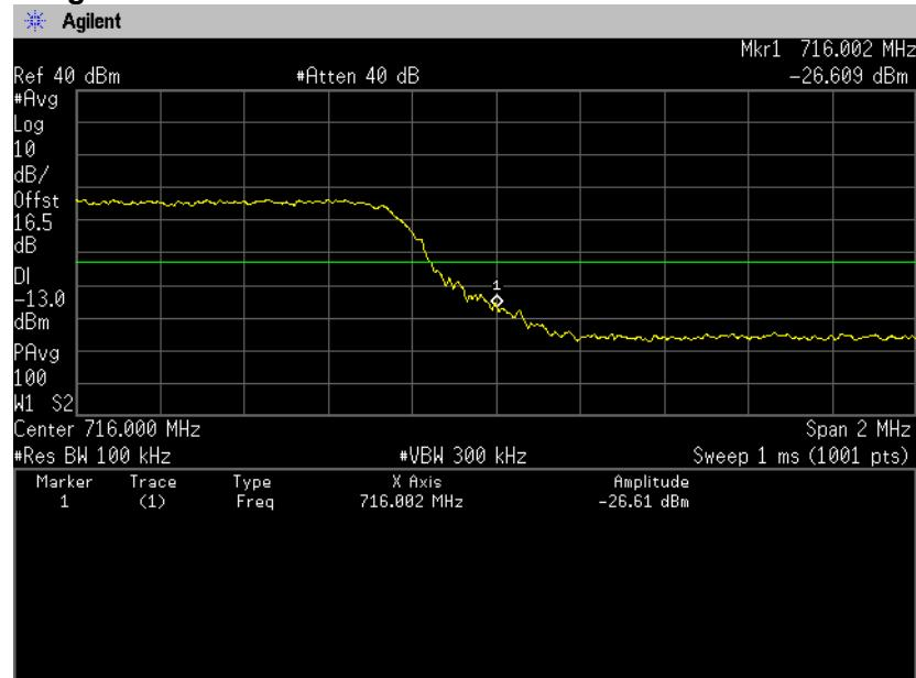
**16QAM, BW 5MHz, RB1-0****Channel: Low**
