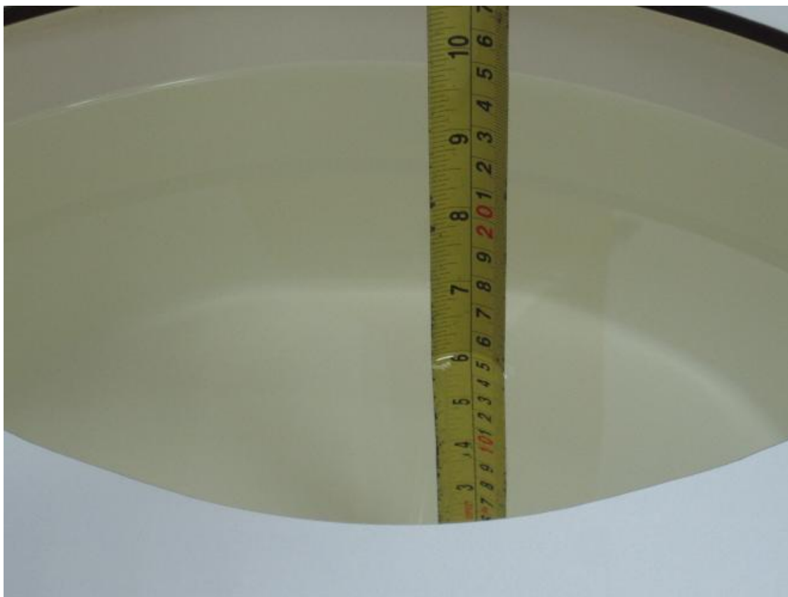
Picture C.3: Liquid depth in the flat Phantom (2450 MHz) (15.2cm deep)
