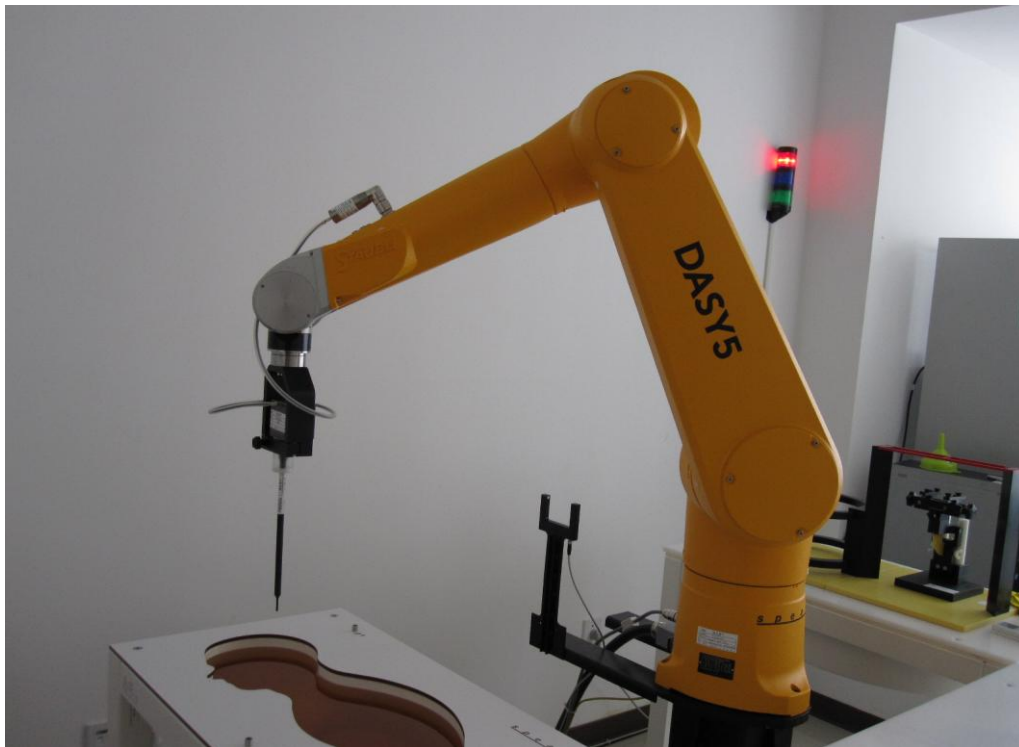
Picture C.1: Specific Absorption Rate Test Layout
