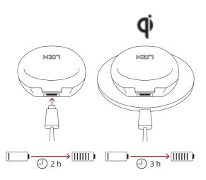
**CAUTION:** Only use the LIZN Charger and USB cable supplied in the box. You can also place the Charger on a wireless charger. Since wireless charging is less efficient, the charging time will typically take 30-80% longer.
