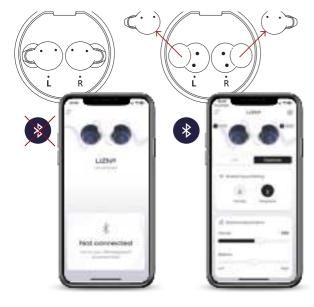
As soon as you remove the two LIZN Hearpieces® from the Charger, your smartphone will detect them and connect by Bluetooth®. NOTE: For first time connection some smartphones require that you connect using the Bluetooth® menu in your smartphone settings to initiate pairing.
