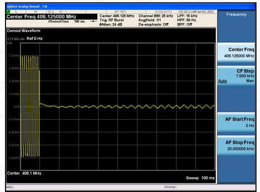
12.5 kHz Channel Separation, Analog modulation, Assigned Frequency:406.125MHz-Turn On
