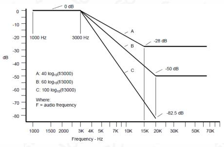
For audio frequencies above 3000 Hz, the audio response of the post limiter low-pass filter shall meet or exceed the following requirements:
