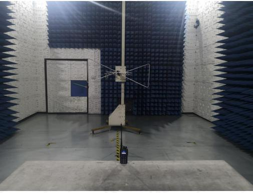
APPENDIX I: PHOTOGRAPHS OF TEST SETUP RADIATED EMISSION TEST SETUP
