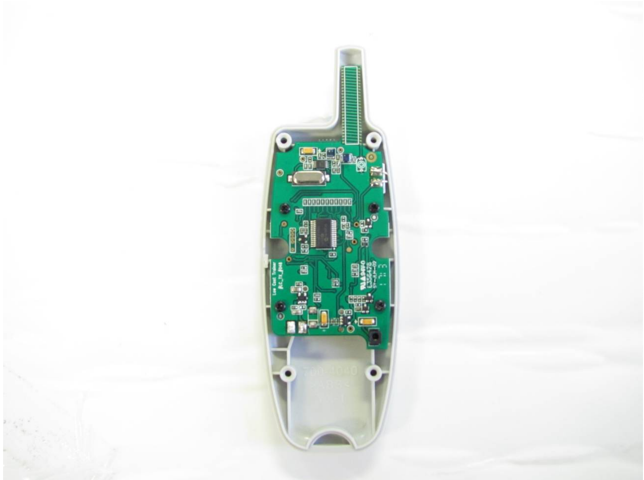
Figure 2. PCB Exposed, Battery Removed
