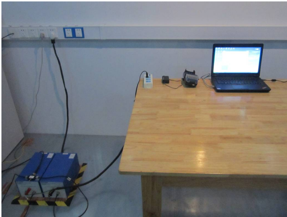
Conducted Emissions Test Setup Front View
