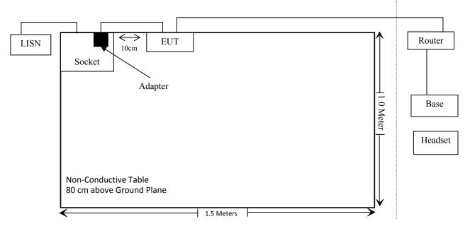
Test Mode2: TX (Powered By POE)
