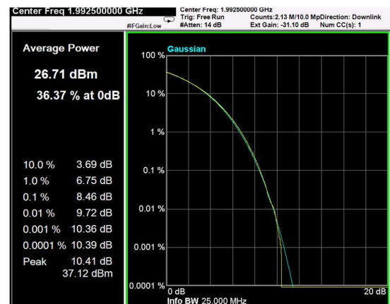
Channel: TOP, Modulation: 64QAM, BW=5MHz, CCDF
