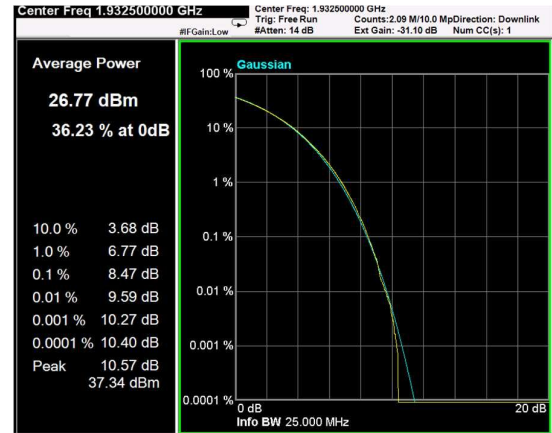
Channel: BOTTOM, Modulation: 64QAM, BW=5MHz, CCDF
