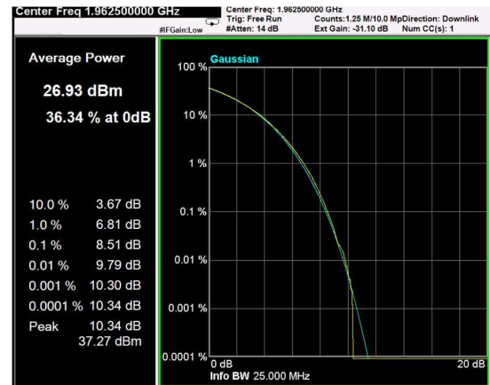
Channel: MIDDLE, Modulation: 16QAM, BW=5MHz, CCDF
