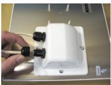
Place Sealing Gasket over screws.
