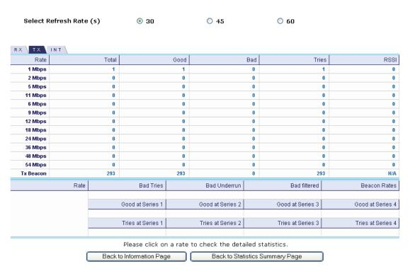
You can click onto each speed level and see how the traffic breaks down. In the TX statistics, there should little to no **Tries at Series 2, 3** or **4**. The radio will try to send a packet 4 times at **Series 1**, and then tries the next series 4 times. In the RX stats, you should look for Bad CRC's and Bad Decrypts for signs of RF interference or Fresnel interference links.
