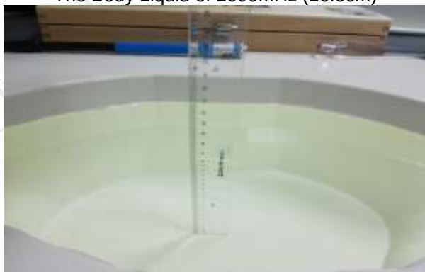
The Body Liquid of 3700MHz (15.2 cm)
