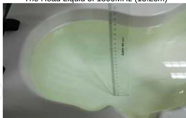
The Head Liquid of 3500MHz (15.3cm)
