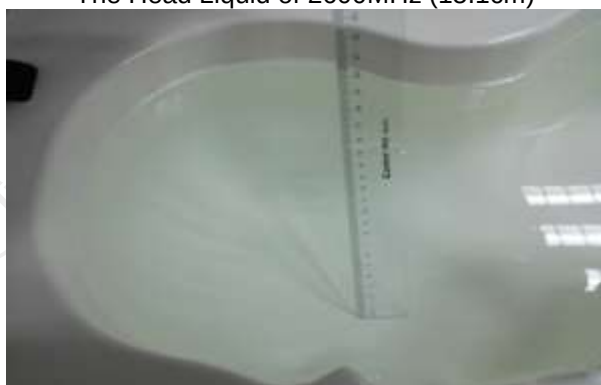
The Head Liquid of 3700MHz (15.6cm)
