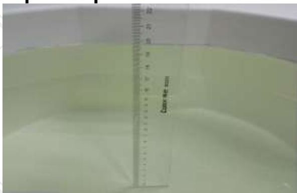
The Body Liquid of 835MHz (15.4cm)
