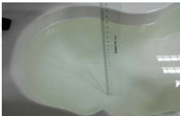
The Head Liquid of 1900MHz (15.5cm)
