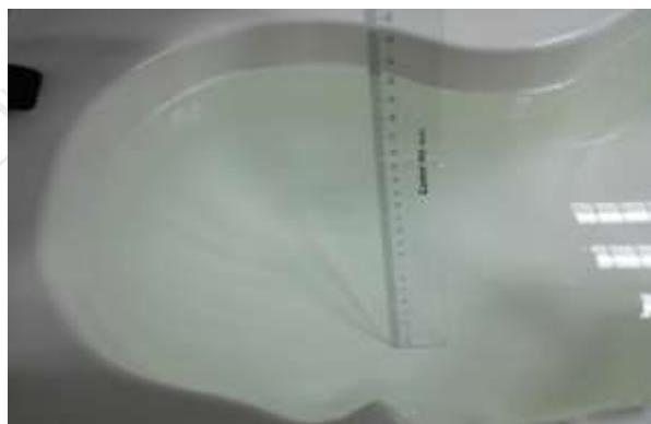
The Head Liquid of 2450MHz (15.6cm)
