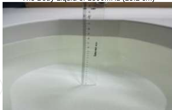
The Body Liquid of 2450MHz (15.3cm)
