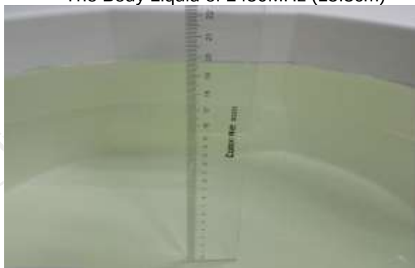
The Body Liquid of 3500MHz (15.4cm)
