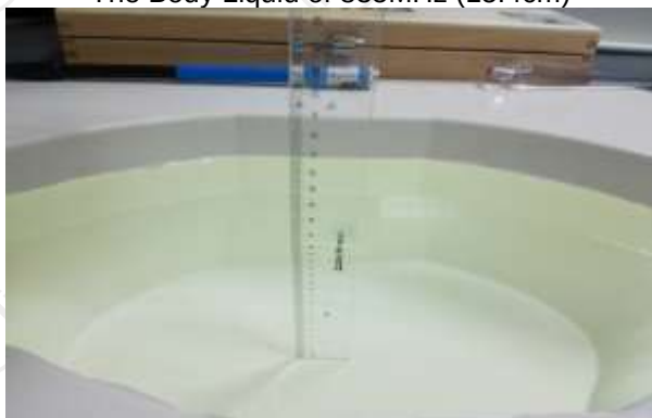
The Body Liquid of 1900MHz (16.4 cm)
