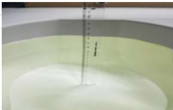
The Body Liquid of 1800MHz (15.2 cm)
