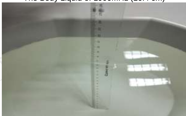
The Body Liquid of 2600MHz (16.5cm)
