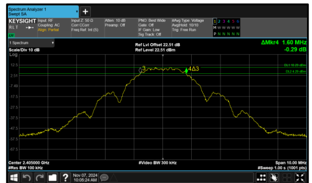
Figure 24 - Core 1 (B) 2405 MHz (CH11) 6 dB Bandwidth
