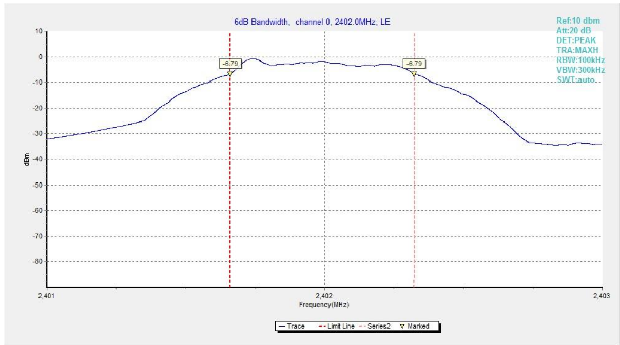
Fig.4 6dB Bandwidth (Ch 0), LE 1M
