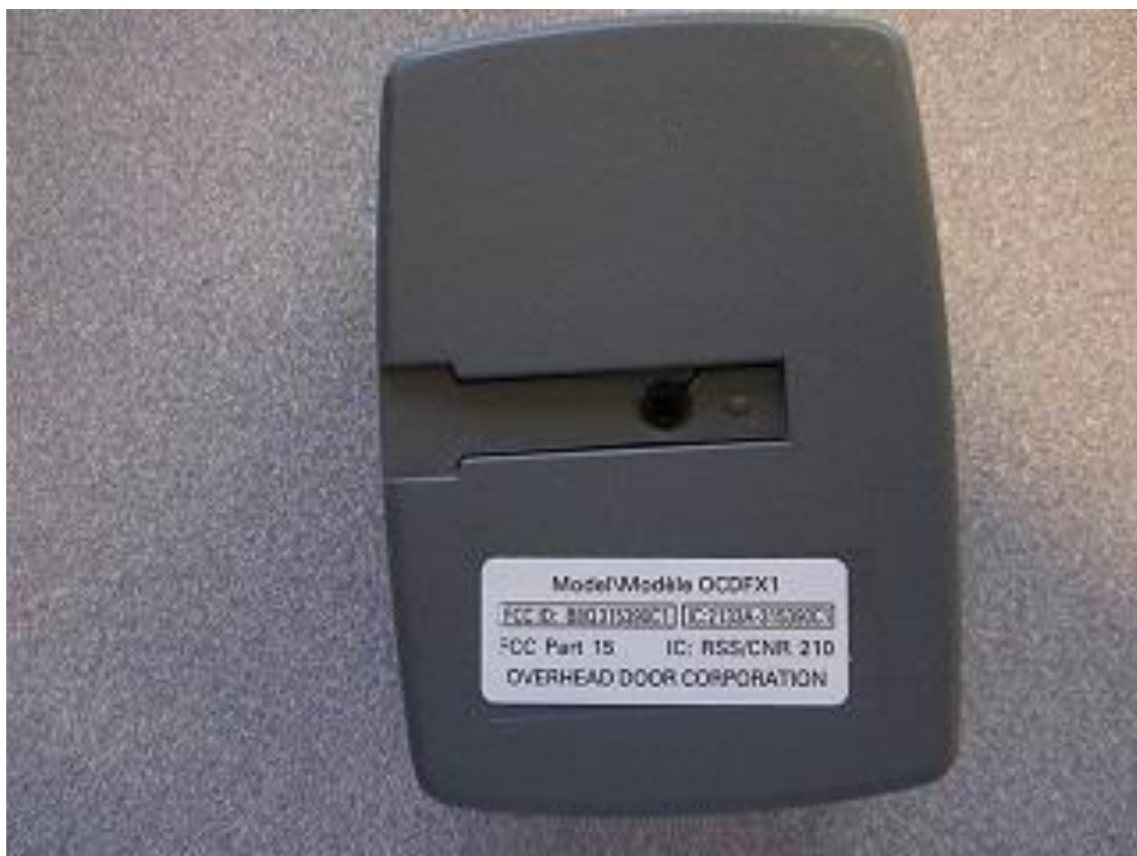
Figure 2: OCDFX1 FCC / IC Label Location
