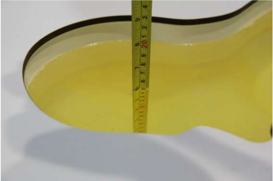
Picture 7-9: Liquid depth in the Head Phantom(2450MHz)
