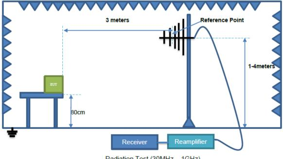
Radiation Test (30MHz - 1GHz)
