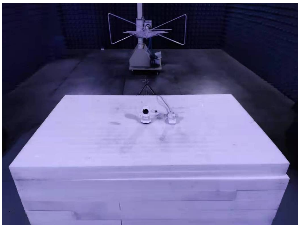
Photo of Radiated Emission Measurement (Below 1G)
