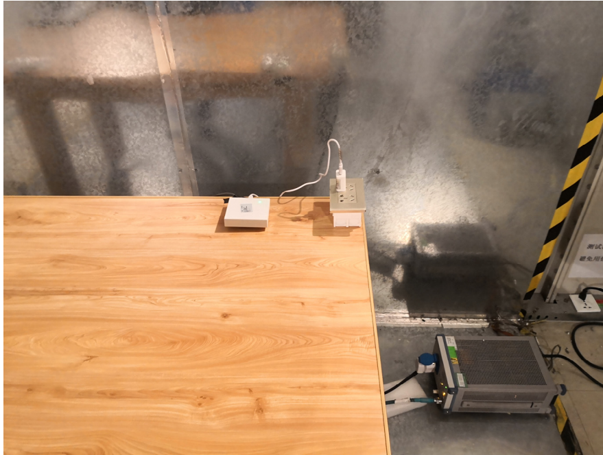
Conducted Emissions (Side View)
