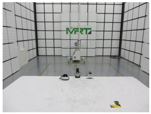
Test Mode: Mode 2 Description: Radiated Emission Test Setup for 1 ~ 18GHz
