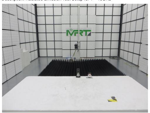
Test Mode: Mode 2 Description: Radiated Emission Test Setup for 30 ~ 1000MHz
