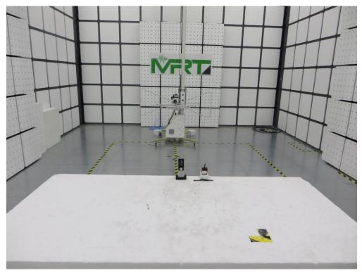
Test Mode: Mode 1 Description: Radiated Emission Test Setup for 1 ~ 18GHz
