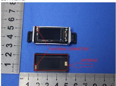
The antenna is integrated on the main PCB and no consideration of replacement. The best case gain of the antenna is -5dBi.
