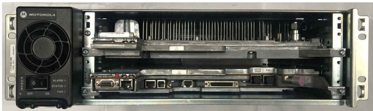
Front View of Base Radio Showing Transceiver Module with TOC Installed and Identifying Connections
