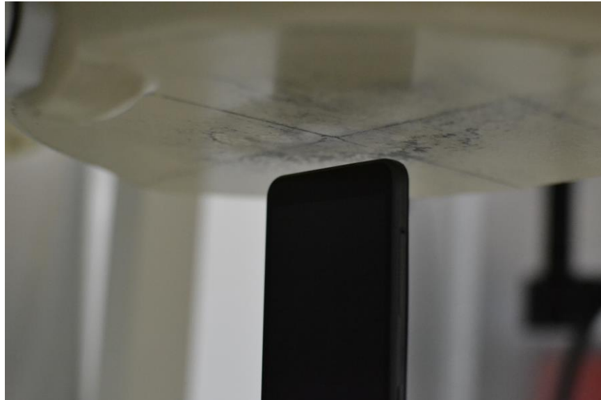
SAR Test Setup Photo 5 – Bottom Edge at 10mm
