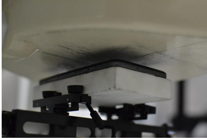
SAR Test Setup Photo 3 – Back Side at 10mm
