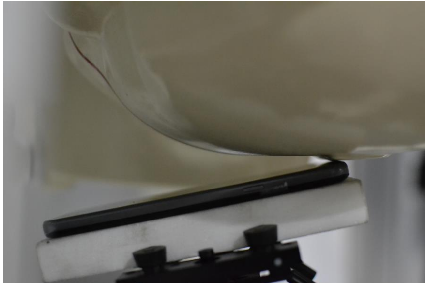
SAR Test Setup Photo – Left Tilt
