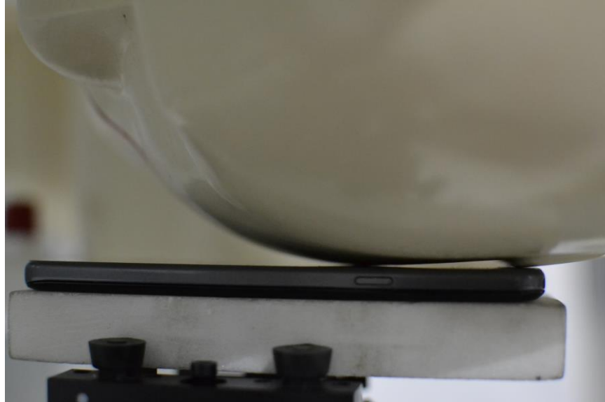
SAR Test Setup Photo – Left Cheek
