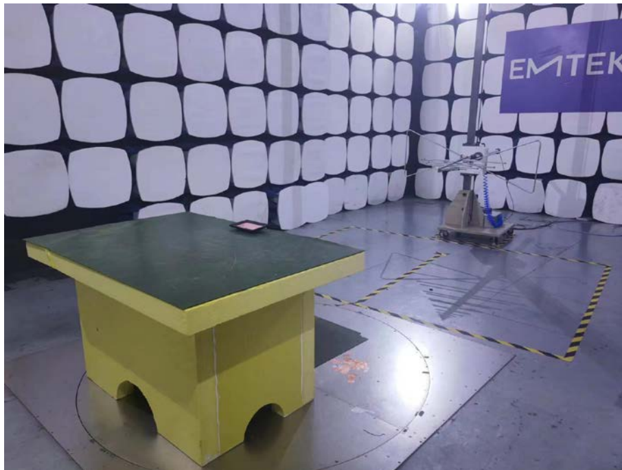
Spurious Emission Test Setup (Below 1GHz)
