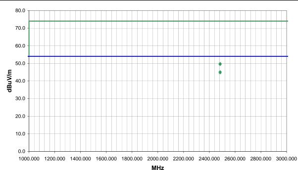
External Distance Compared to Freq Amplitude Factor Azimuth Distance Polarity Adjusted Spec. Limit Height Detector Attenuation Adjustment Spec. (dBuV) (dB) (meters) (dB) (dB) dBuV/m dBuV/m (dB) (degrees) (meters) (MHz) 23.6 227.0 1.0 3.0 H-Horn ΑV 45.2 54.0 2483.689 1.6 20.0 0.0 -8.8 2483.549 23.1 1.6 79.0 1.0 3.0 20.0 V-Horn AV0.0 44.7 54.0 -9.3 2483.880 28.3 1.6 227.0 1.0 3.0 20.0 H-Horn PΚ 0.0 49.9 74.0 -24.1 2483.560 27.8 1.6 79.0 1.0 3.0 20.0 V-Horn PΚ 0.0 49.4 74.0 -24.6
