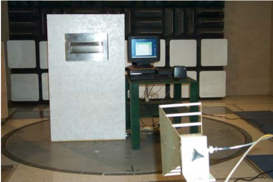
TEST SETUP Radiated Emissions 1 to 10 GHz
