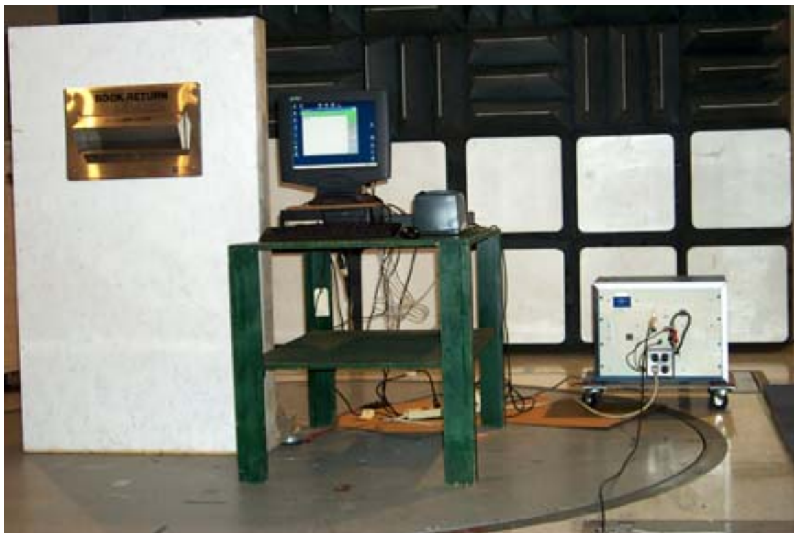
TEST SETUP Conducted Emissions
