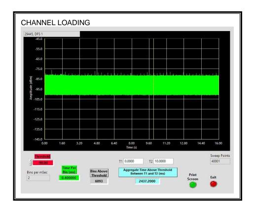
The level of traffic loading on the channel by the EUT is 24.37%
