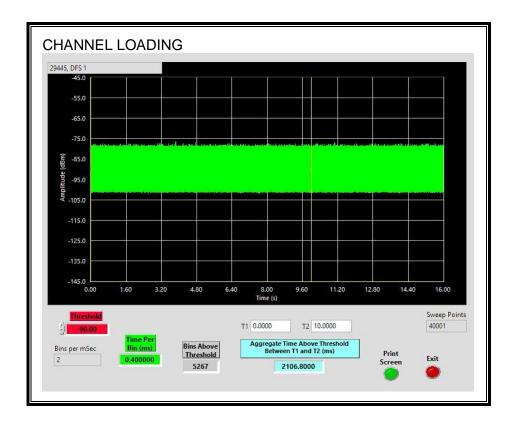
The level of traffic loading on the channel by the EUT is 21.06%
