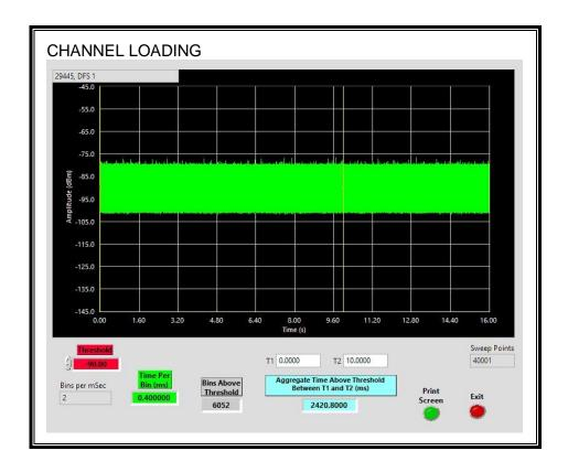
The level of traffic loading on the channel by the EUT is 24.2%
