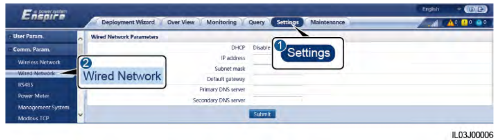
Figure 6-8 Setting wired network parameters
