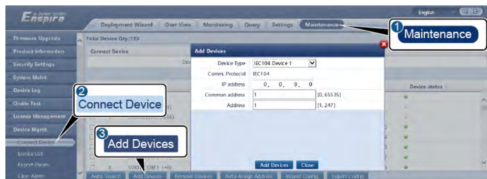
Figure 6-40 Setting access parameters
