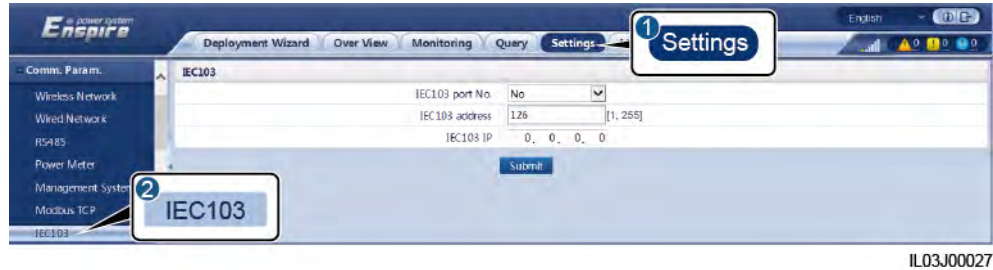
Figure 6-32 Setting IEC103 parameters
