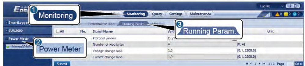
Figure 6-23 Setting running parameters
