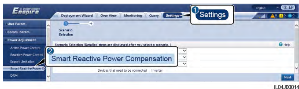
Figure 6-47 Setting parameters for smart reactive power compensation.
