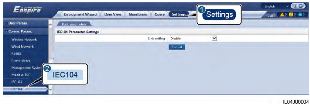
Figure 6-11 Setting IEC104 parameters
