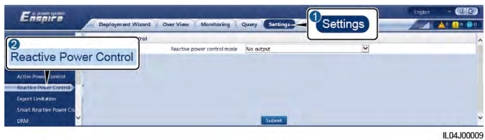
Figure 6-43 Reactive power control
