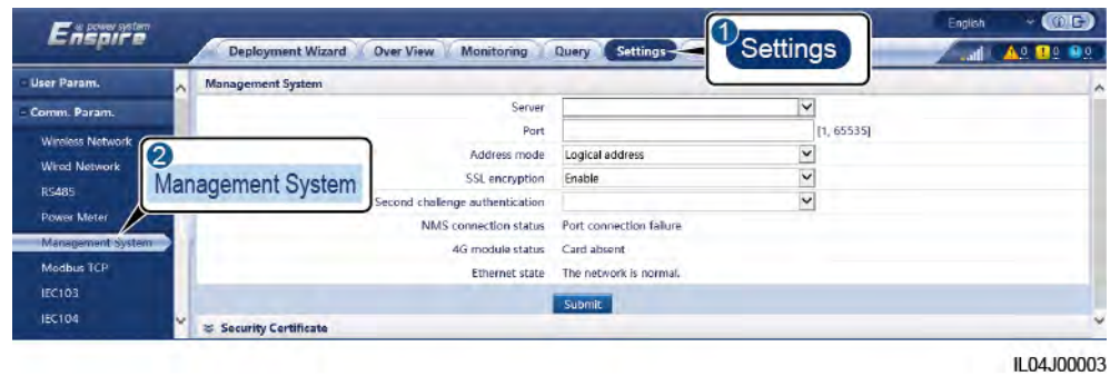
Figure 6-9 Setting management system parameters
