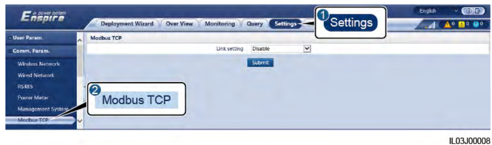
Figure 6-10 Setting Modbus TCP parameters
