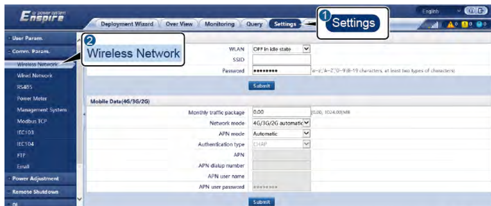
Figure 6-7 Setting mobile data parameters
